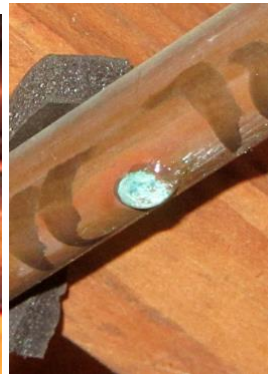
Corrosion with water dripping.
